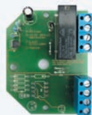
Relays* to control ancillary equipment
